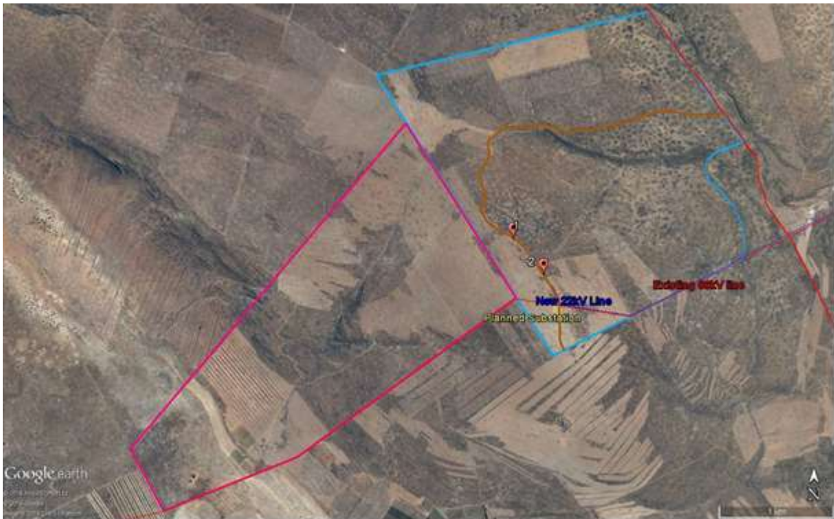
Figure 3: The revised layout of two turbines (2016), the existing 66kV power line running along the southern boundary of the site in pink with a short 22kV line connection to the substation in yellow. The access road is in orange.
