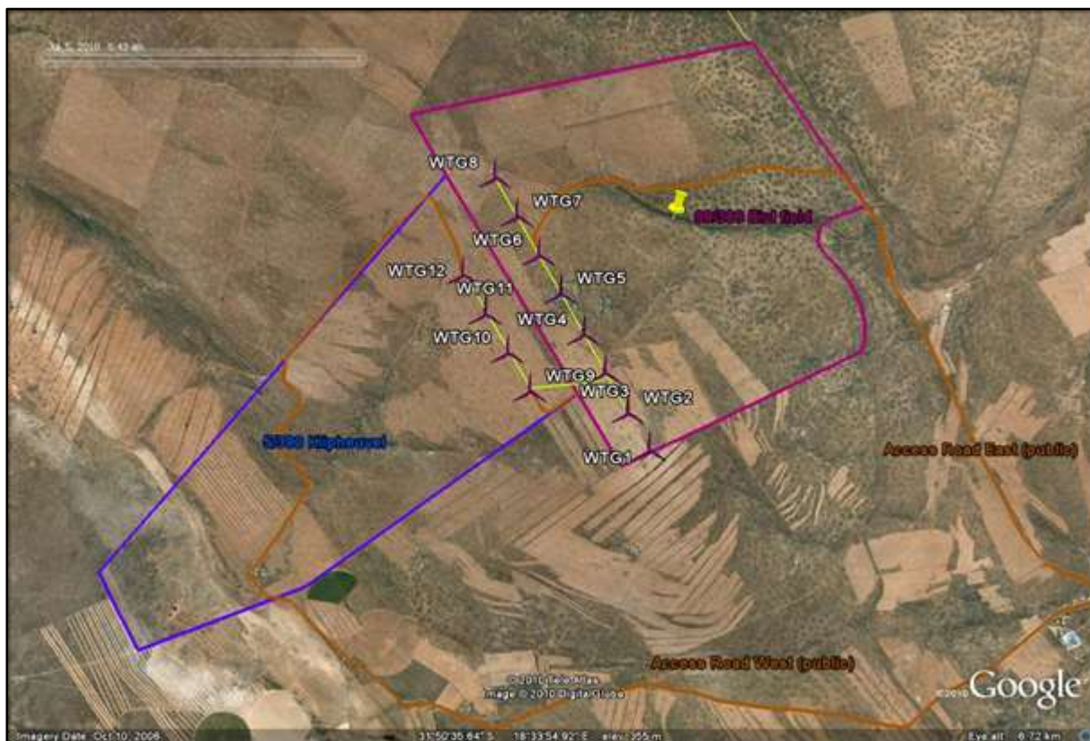
Figure 2: The original layout of twelve turbines (2011), the proposed access roads, substation and underground electrical cable on Klipheuel and Bird Field.
