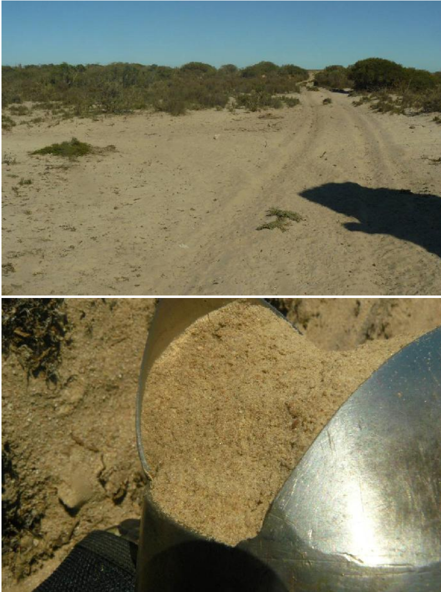
Photograph 3: Cohesionless quartzite sands which dominate the project site
