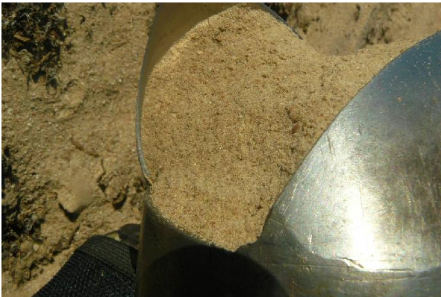
Photograph 3: Cohesionless quartzite sands which dominate the project site
