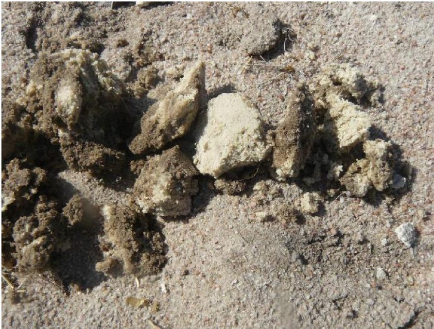
Photograph 2: Saturated soft carbonate horizon
